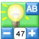
**BRIGHTNESS** CLICK the BUTTON for auto brightness. Use the and BUTTONS to manually adjust brightness. When Auto Brightness is active, the value in the BUTTON WINDOW is "Gray".
