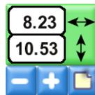
**SCAN SIZE** Use the and BUTTONS to manually ADJUST the SCAN SIZE. CLICK the AUTO-ADJUST BUTTON to automatically ADJUST the SCAN SIZE. When AUTO-ADJUST is active, the dimensions shown on the BUTTON WINDOW are "Gray".
